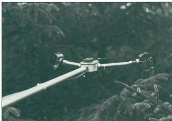
Sensitive three-axis anemometer for windspeed and turbulence measurements. (Constructed in the Forestry Commission Research Workshop.)
