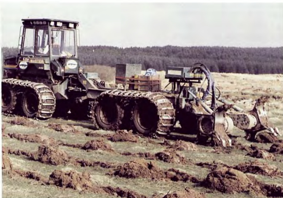
Donaren 2-row continuous moulder mounted on an OSA 280 Master forwarder.
