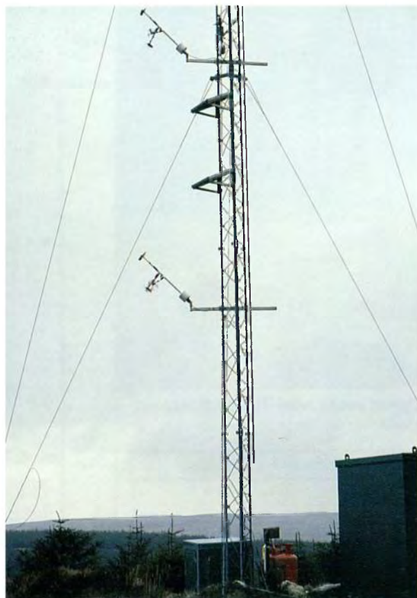
Three-axis anemometers for obtaining turbulence information during the Kintyre airflow study.
