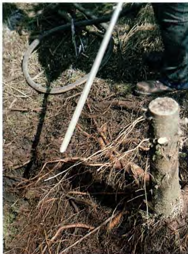
Supersonic air knife used to expose tree roots (C. P. Quine)
