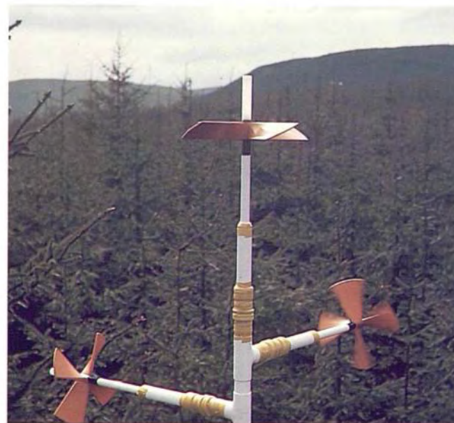
Anemometers in place over 11 m high Sitka spruce plantation.
