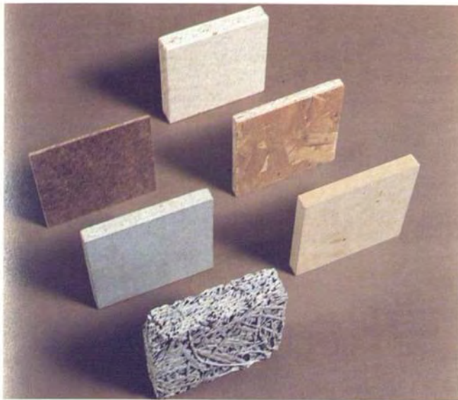
Wood-based panel products. Clockwise from top: wood chipboard, oriented strand board, medium density fibreboard, wood wool cement slab, cement bonded particleboard, hardboard (a fibre building board).
