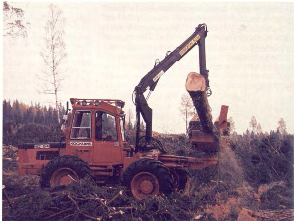
Bed processor working on clear felling.
