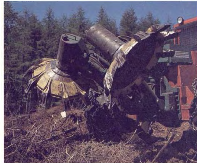
Disc trencher on restock site.
