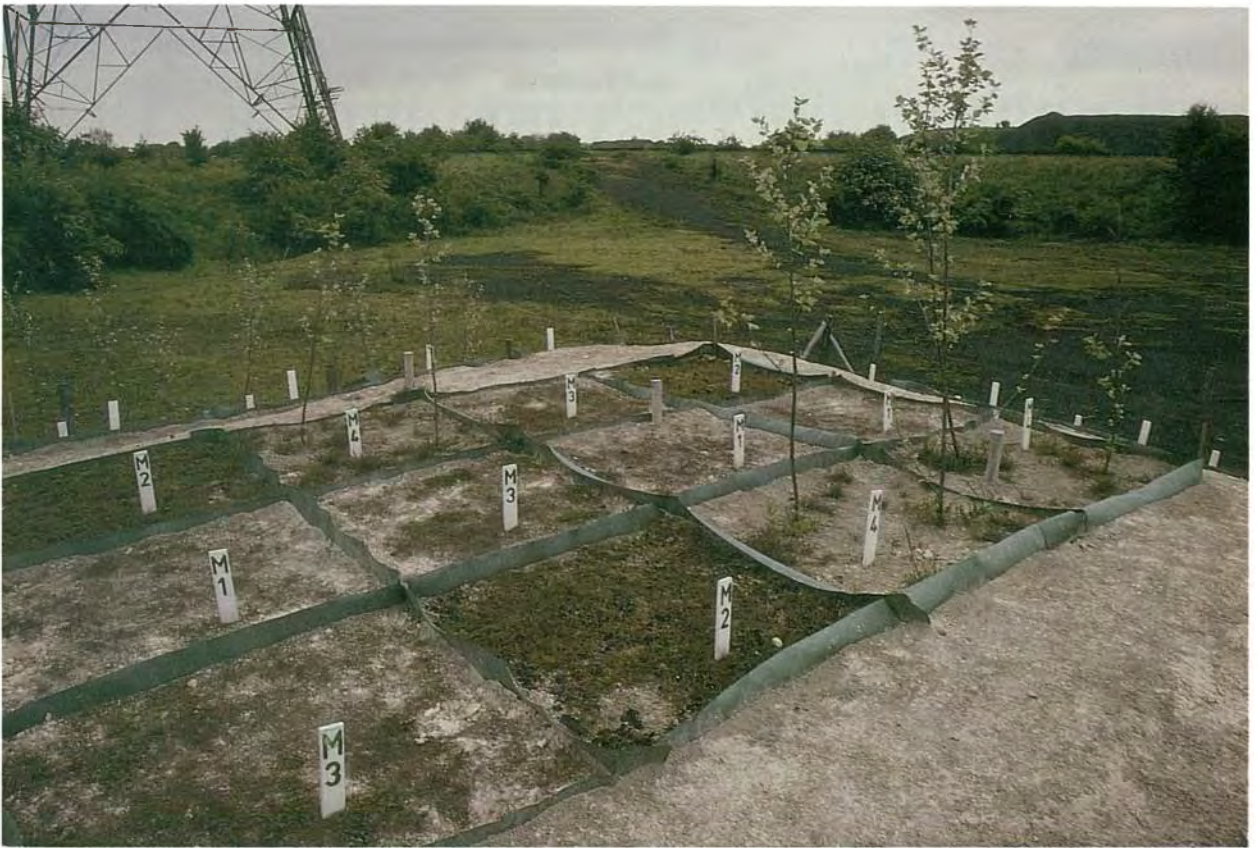
Plate 6 An experiment established at West Burton Power Station to investigate the establishment of white poplar on a gypsum mound; trees planted in M4 plots only. (I. Collier).
