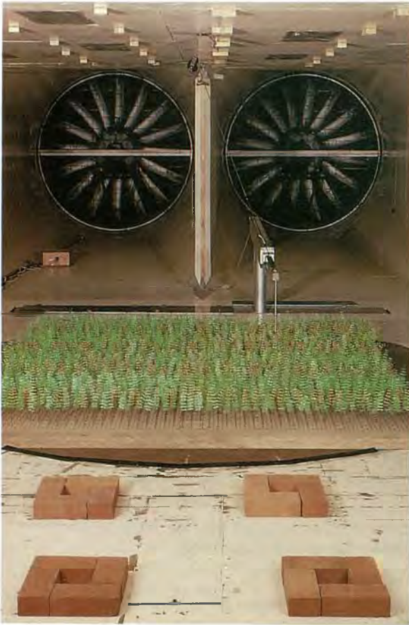
Plate 4 Model trees in the wind-tunnel at Oxford University. (39288).
