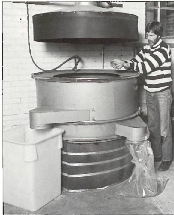
Figure 9.6 Vibrating separator used at Alice Holt for dewinging seeds. (B9394).
