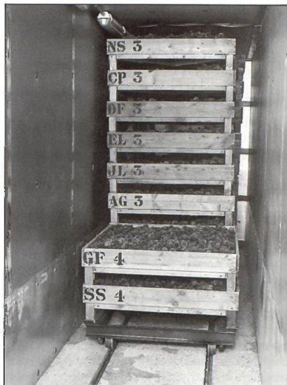
Figure 9.3 The tunnel stage of the Alice Holt kiln. (B9392).
