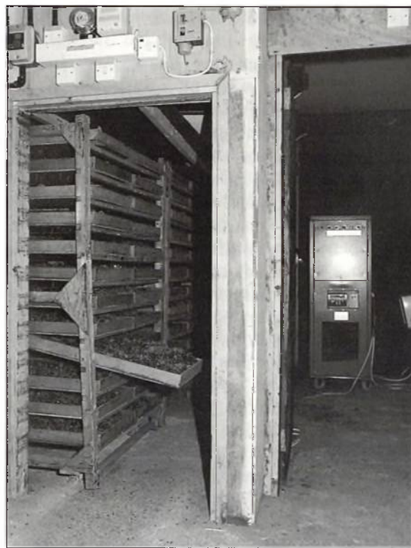
Figure 9.5 Forestart kiln using heat pump as source of cheap and efficient energy. (Photo: John Poole Photography).
