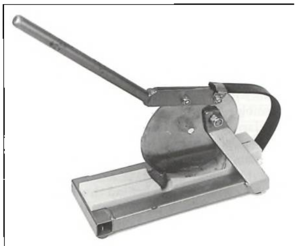
Figure 7.1 New Canadian designed cone cutter (F.D. Barnard, P.O. Box 144, Blind Bay, B.C., Canada, V0E 1H0). (Photo: John Poole Photography).
