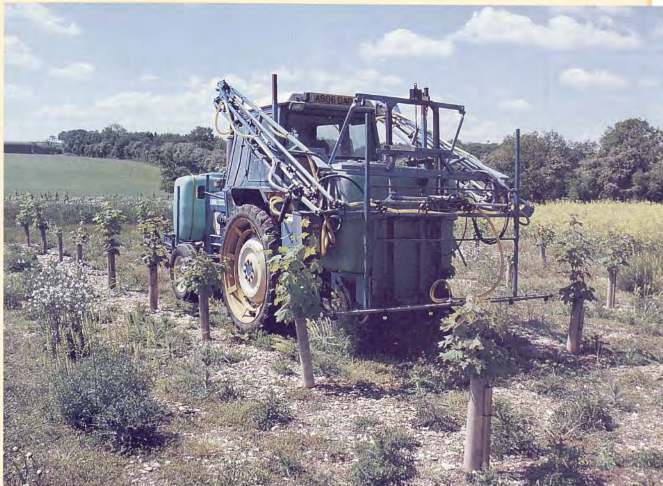
PLATE 18 A normal agricultural sprayer adapted by the addition of a short boom on the rear of the sprayer for use in farm woodlands. (40156)
