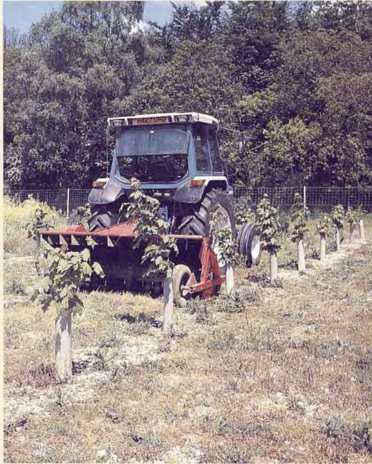
PLATE 14 Mechanisation of mowing the inter-row vegetation. Residual herbicides were used to control weeds along the tree rows. (40158)
