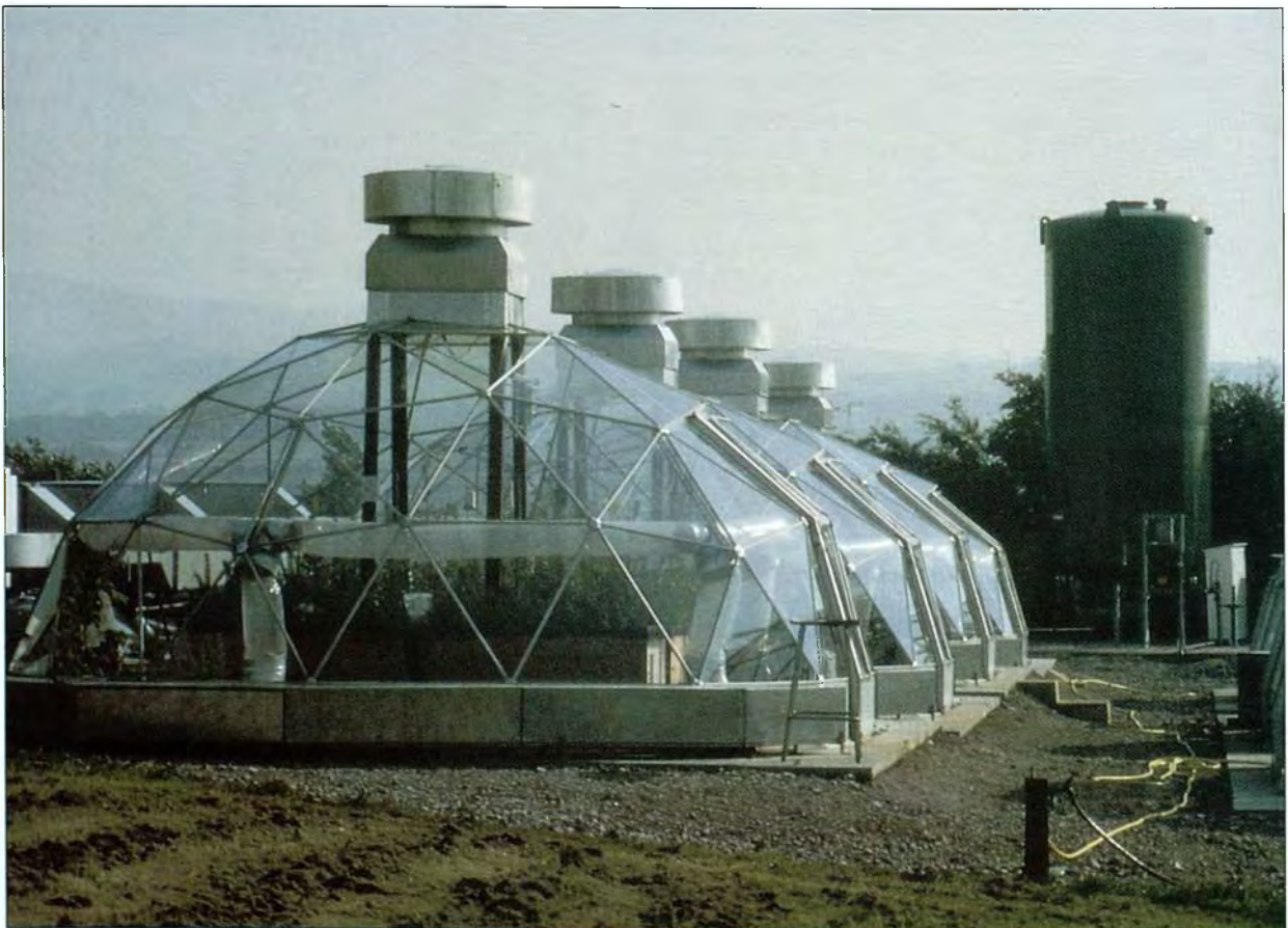
Plate 8. The solardomes and CO 2 tank at the Biology Field Station, Lancaster University.
