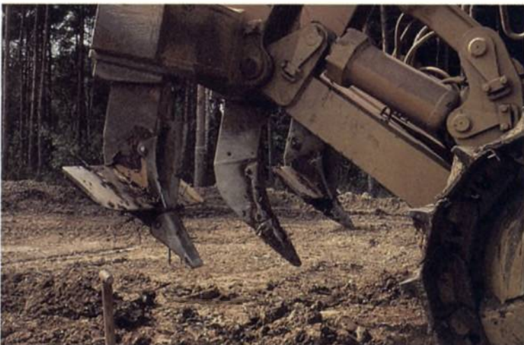
Plate 20 Tine assembly on a Caterpillar D8 (300hp); the two outer tines are winged; depth of working 750 mm.
