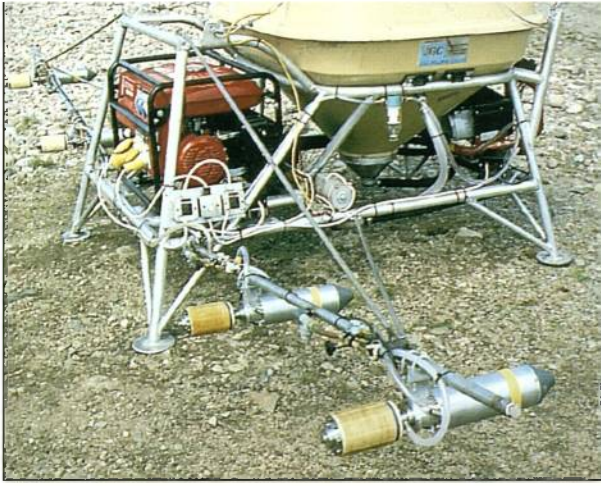
Plate 1. The self-contained, ultra low volume application system developed by Entomology Branch for controlled droplet application of pesticides to forests.
