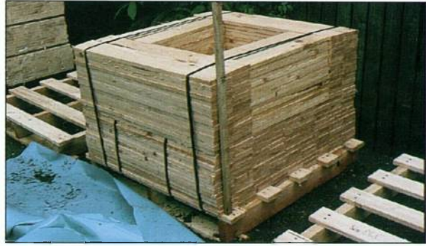
Plate 6. Freshly sawn close-stacked pine lumber constructed in a nest arrangement, just before the addition of plastic tanks containing sterilised board samples to the central part of the stack.
