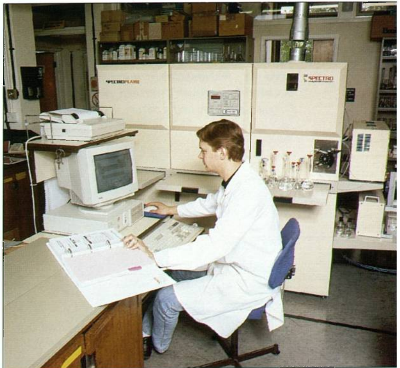
Plate 4. Inductively coupled plasma spectrometer for analysis of major and minor nutrients.
