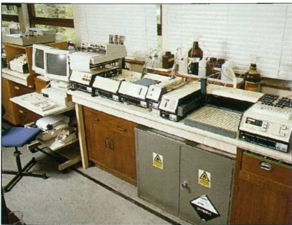
Plate 3. Continuous flow systems for analysis of nitrogen and phosphorus.
