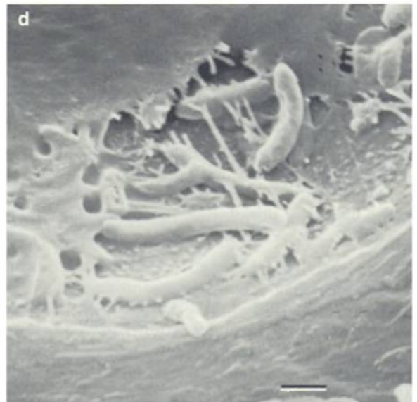
Plate 13 Scanning electron micrographs of bordered pits in softwood tracheids showing (a) intact pit from freshly felled Scots pine log and (b)-(d) bacterial degradation of the torus (t) and margo (m) in pits from a c. 4-year wet stored log. Bar lines for (a) and (b) are 10 \mu\text{m} , (c) and (d) are 1 \mu\text{m} . (VANESSA CLARK)
