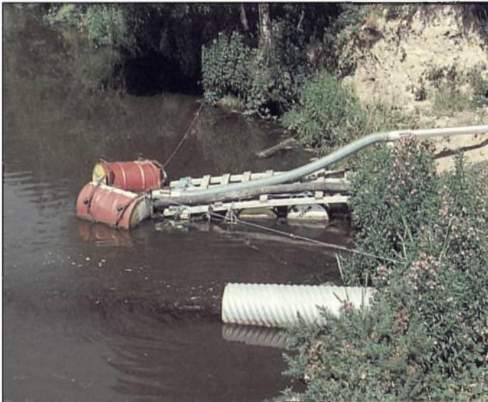
Plate 6 Point of water abstraction (background) from the gravel pit for irrigating the wet store and point of return (foreground) for the coloured effluent draining from the site.
