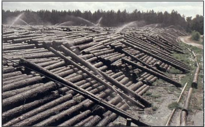
Plate 1 Western end of wet store showing the security logs in place. (38804)
