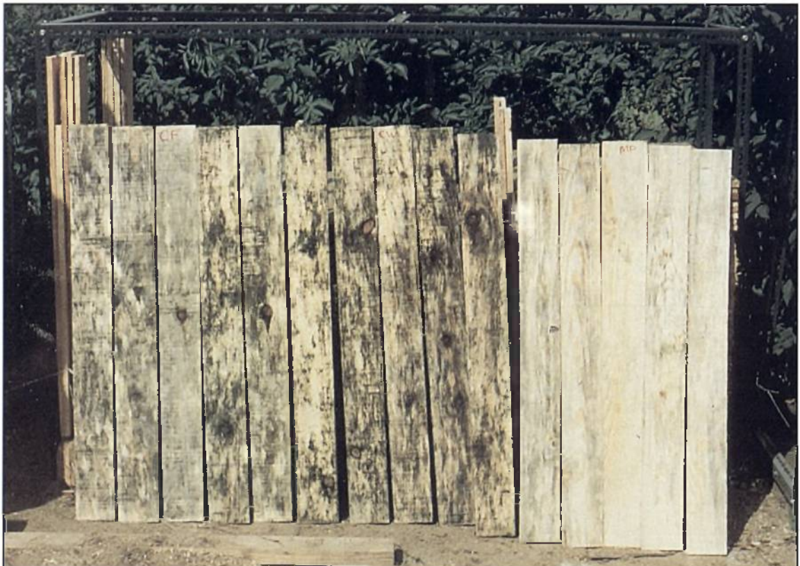
Plate 12 Susceptibility of five replicate boards cut from freshly felled logs (left), 6-month water stored (centre) and c. 4-year water stored logs (right) exposed in stacks for 8 weeks. (MICHAEL POWELL)
