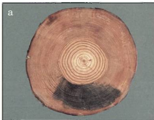
Plate 10 Cessation of development of pre-existing bluestain in water stored pine. (a) Section cut 5 cm from the end of a Corsican pine log showing the same amount of bluestain after 21 months as was recorded when the log went into store. (39331) (b) Section cut 25 cm from the end of the same log showing a little discoloration but no bluestain. (39332)
