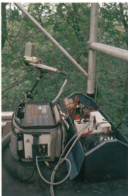
Figure 10. Physiological characterisation of a mature oak stand. Portable gas-exchange analysis system (LCA-3: ADC Ltd.) used to parametrise photosynthesis and transpiration profiles.
