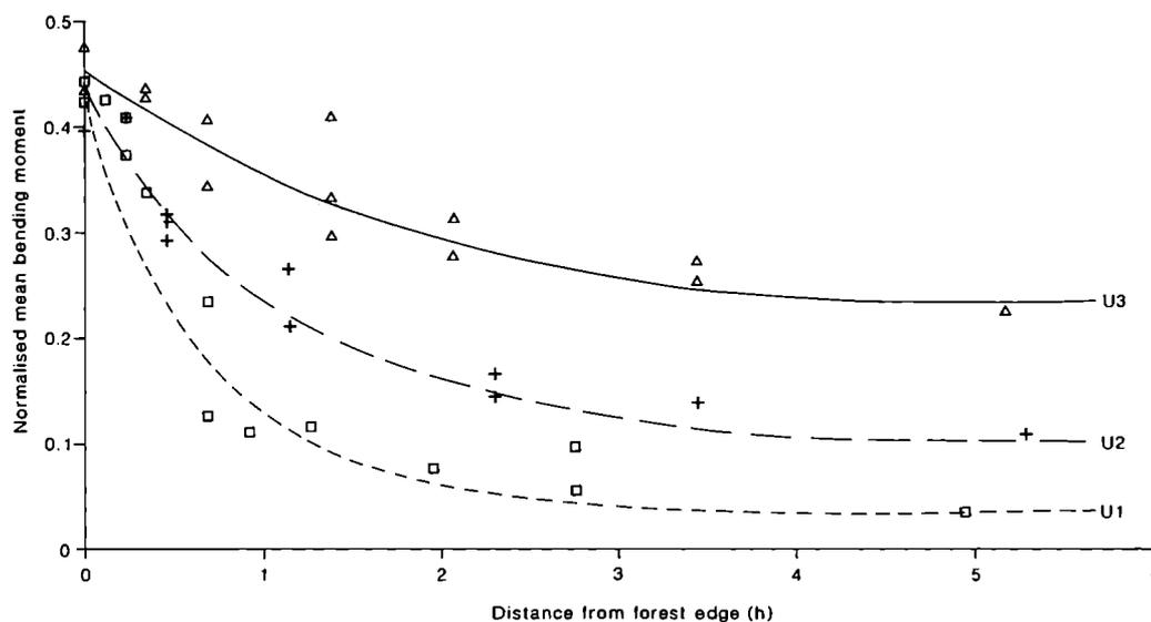
**Figure 3a** Normalised mean bending moments at different distances (in tree heights) back from the untreated edge of forests with different planting densities (U1 = 1.7 m spacing, U2 = 3.5 m spacing and U3 = 5.2 m spacing). All bending moments are normalised by dividing them by the extreme bending moment at the untreated edge of a forest with standard spacing (U1) to allow easy comparison between treatments.
