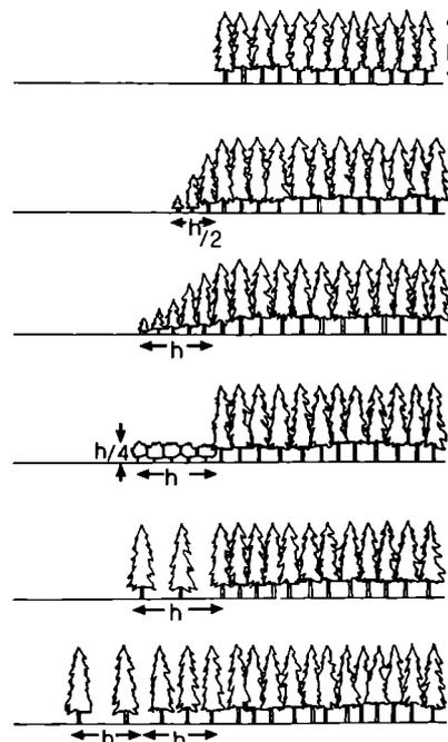
**Figure 1** Designs of forest edges tested in the wind tunnel, where  $h$  represents mean tree height.
