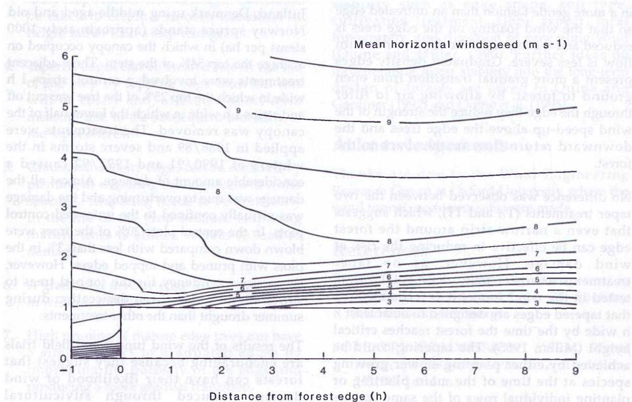
**Figure 5** Contours of mean wind speed across an untreated forest edge (U1). Note the increase in wind speed just above the edge trees.
