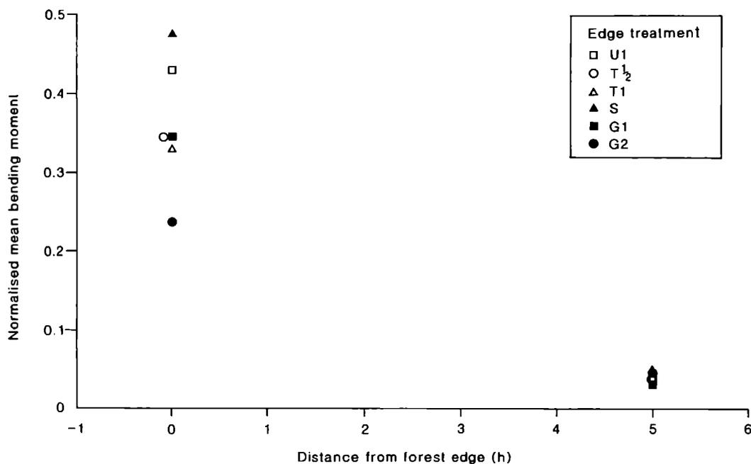
**Figure 4a** Normalised mean bending moments at the forest edge and 5 tree heights back from the edge for different edge treatments. As in Figures 3a and 3b, all bending moments are normalised by dividing through by the extreme bending moment at the untreated edge of a forest with standard spacing (U1). See Figure 1 for explanation of symbols.
