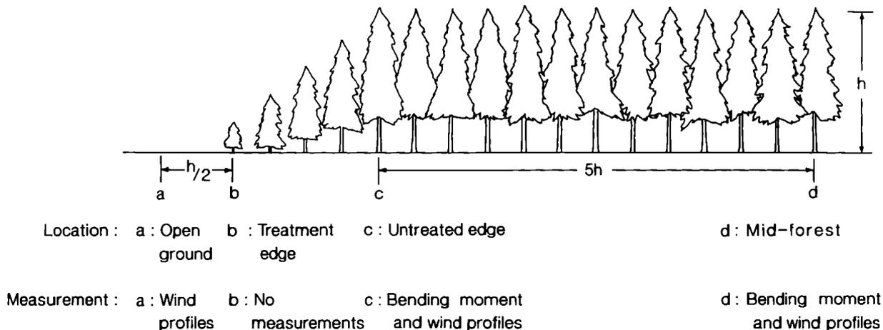
Figure 2 Types and positions of measurements in relation to the treated forest edge.
