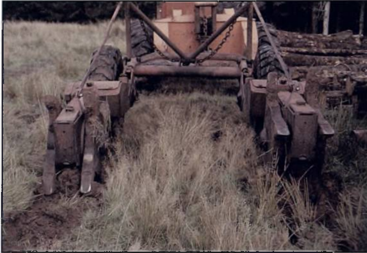
Plate 10. A Brücke patch scarifier preparing intermittent planting spots on a moist brown earth site with light grass cover. (38644)
