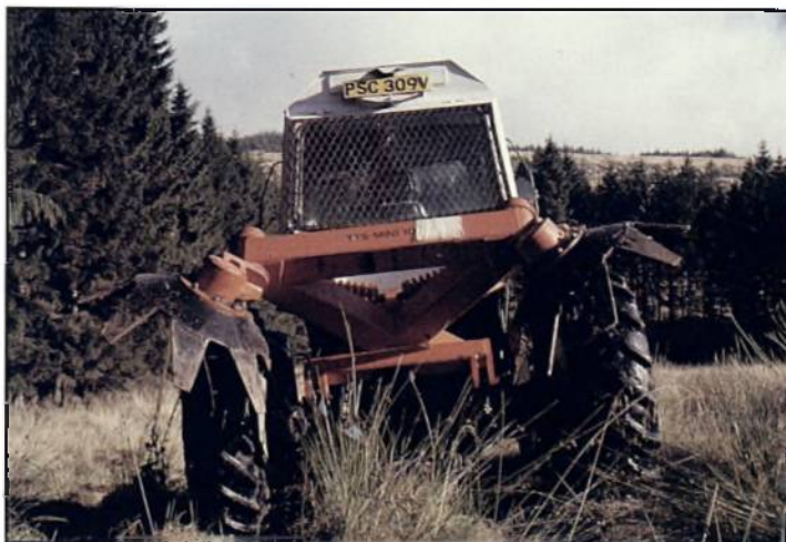
Plate 3. The lighter TTS-10 scarifier used to bare the mineral soil surface on podzols and brown earths. The discs are not powered. (38635)
