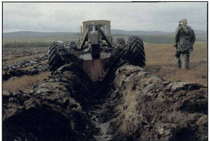
Plate 8. A double mouldboard trailed plough preparing an afforestation site on deep peat in Shin Forest in north Scotland in the late 1970s. This is deep cultivation at a depth of around 60 cm.
