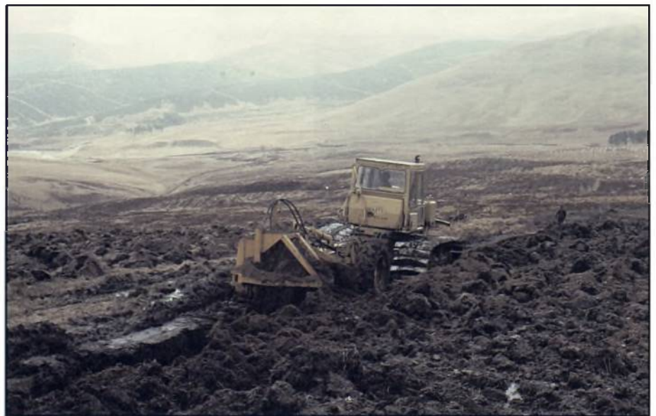
Plate 25. The prototype rotary mouldboard plough carrying out complete ploughing of an afforestation site on a peaty ironpan soil in the Moffat hills in south Scotland.
