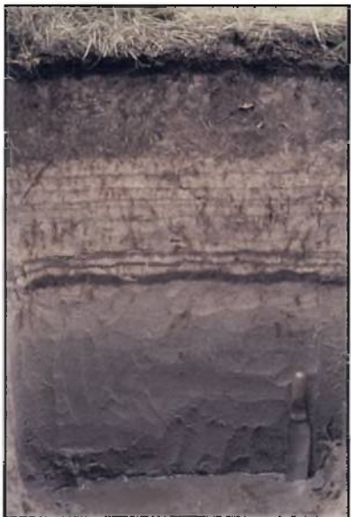
Plate 15. A sandy littoral soil with a shallow water table (type 15g) from Roseisle Forest near Elgin in north-east Scotland. Cultivation should provide a raised planting position through mounding to reduce the frost risk and provide all round stable rooting.
