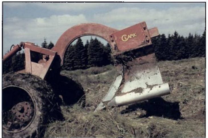
Plate 6. A prototype deep mole plough used in a number of restocking experiments in the late 1970s and early 1980s. The mole comprises a 25 cm diameter oxygen bottle welded on to the base of a drainage plough with a 10 cm tine sock. The mole was created at depths of 60–90 cm.
