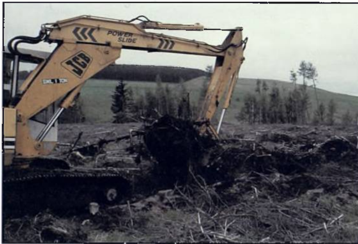
Plate 5. A tracked excavator being used to prepare mounds on a peaty gley restocking site in Kielder Forest. A mounding bucket would be preferable to the drainage bucket shown here.
