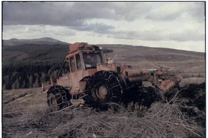
Plate 7. A TTS-35 Delta scarifier with powered discs mounted on the back of a modified Timberjack skidder. (38651)
