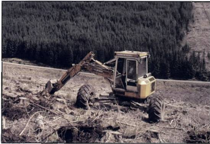
Plate 1. A Menzi Muck walking excavator preparing mounds on an upland brown earth restocking site in Argyll. (51200)
