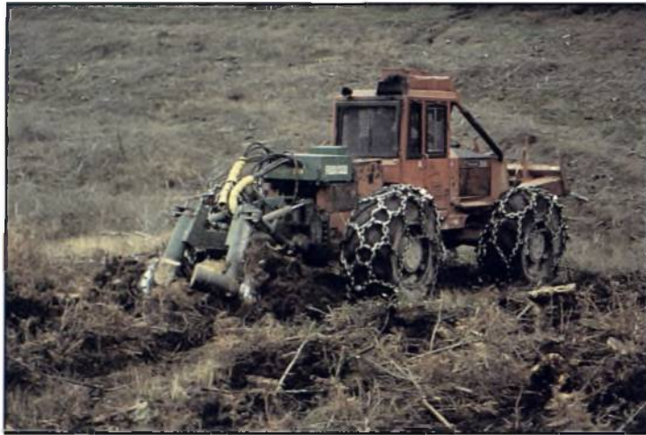
Plate 4. A Donaren 280 scarifier working in the disc trench setting on a restocking site on an upland brown earth soil in North Wales. The discs on this machine are powered.
