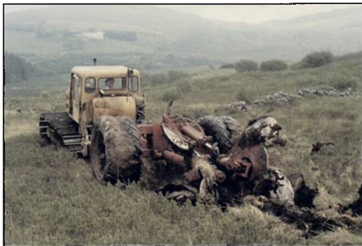
Plate 9. A Maclarty moulder working on a flushed peat afforestation site in south-west Scotland.
