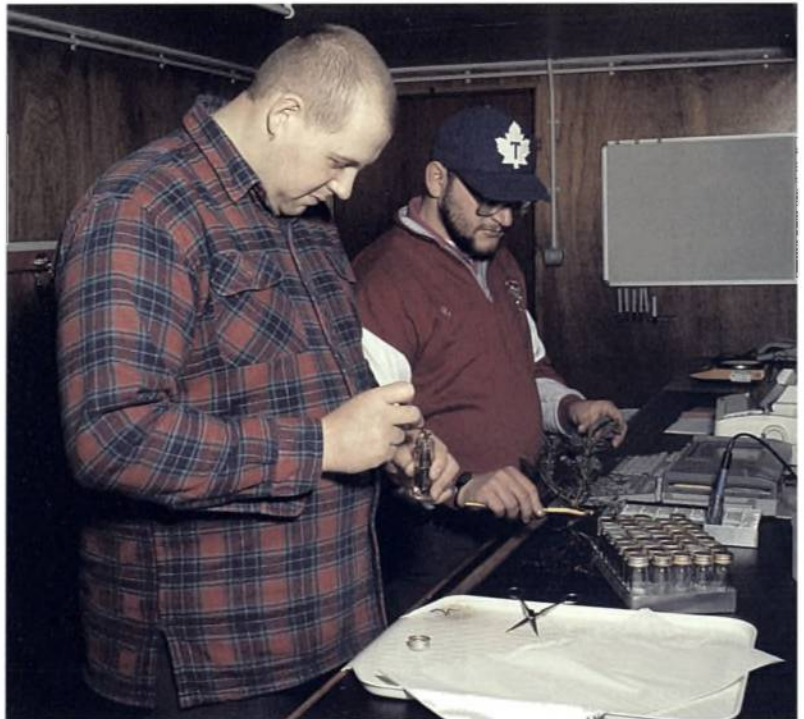
Plate 19 Plant quality testing laboratory at Bush nursery. Plants are routinely tested for RGP, electrolyte leakage and root moisture content. Physical measurements compare plants against British Standards. (51221)
