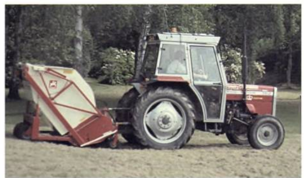
Plate 27 Forage harvesters may be used to cut and collect vegetation on sites where build-up of nutrients may pose a threat to floristic diversity. (R. FERRIS)
