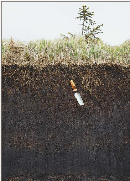
Figure 3 This soil is clearly classed as a Deep peat because the humus depth is greater than 45 cm.
