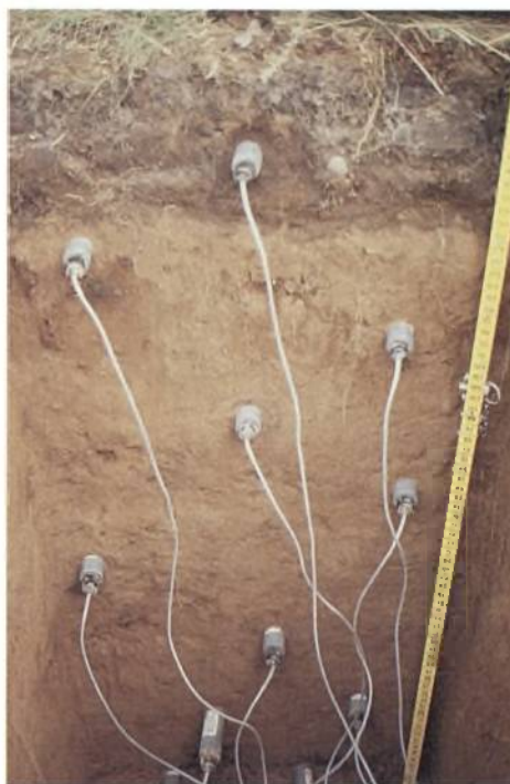
Figure 5.9 Soil moisture probes are being employed in Clipstone Forest in Nottinghamshire, along with other techniques, to compare the water use by oak, Corsican pine, heath and grass.
