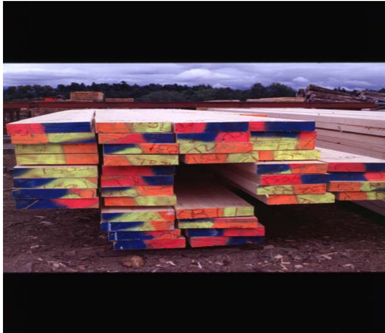
Plate 8 The final battens illustrating the markings which allow identification of their origin.
