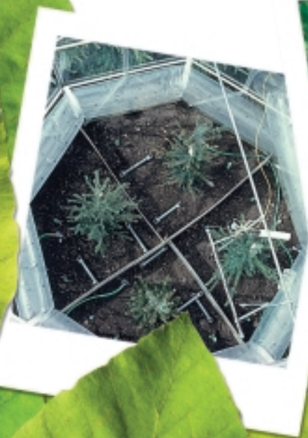
Open-top chamber used for air pollution and climate change research
