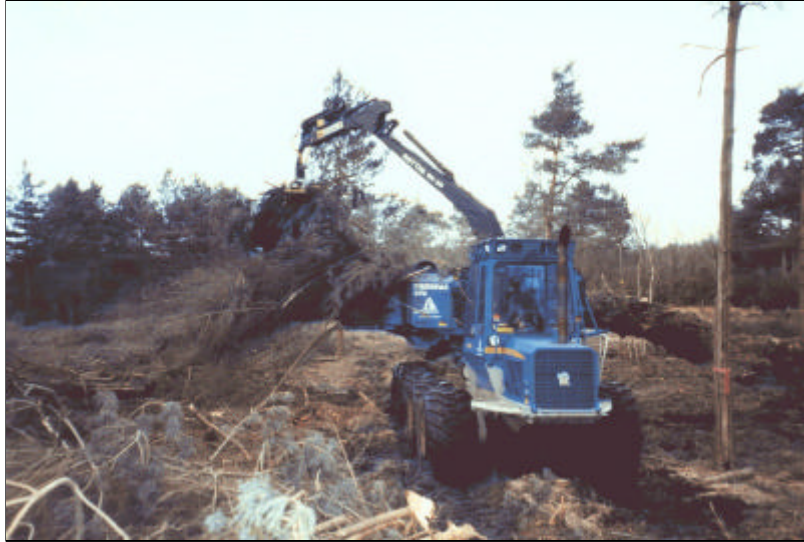
Plate 2. Bailing brush for fuel wood burning. Well-presented brush aids the process. Note the ground impact of the machine, typical for large-scale forest machinery
