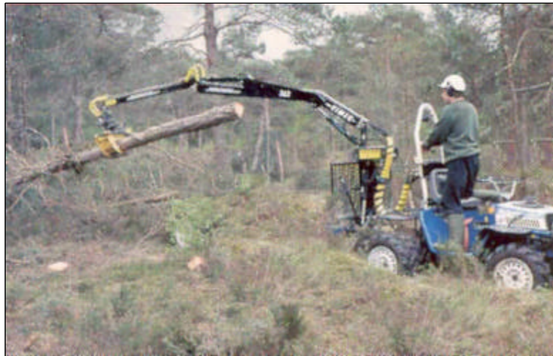
Plate 1. Mini Forwarder Extraction of whole trees from a bog habitat restoration site by a Vimek Minimaster
