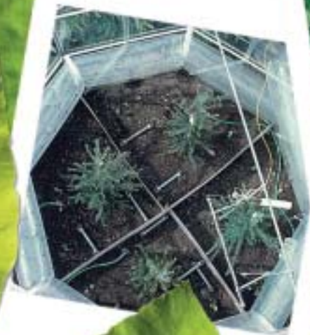
Open-top chamber used for air pollution and climate change research
