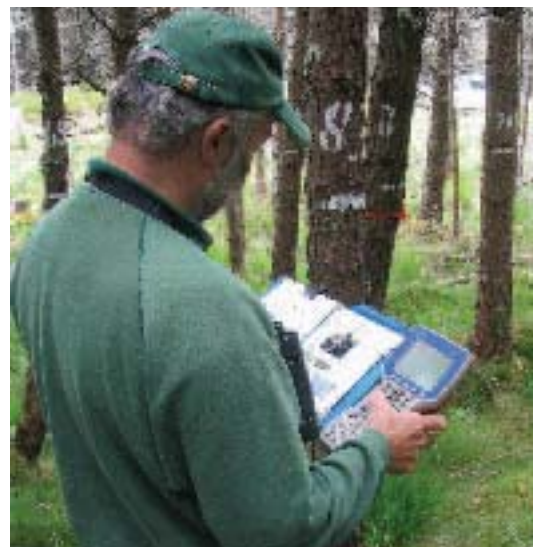
Surveyors record FCS assessments using hand-held computers which provide context-sensitive help and carry out data consistency checks in the field.
