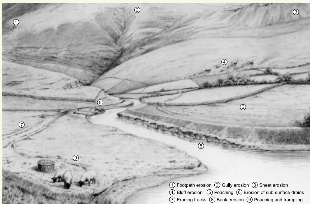
Figure 3 A 3-d diagram depicting the movement of sediment along the source-receptor pathway in the catchment of Bassenthwaite Lake.
