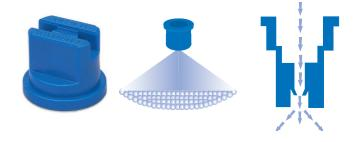
Off-centre even flat fan nozzles can be used to apply herbicide to the side of a tree which is a safer alternative to over-spraying. This enables weeding to take place when the tree is taller than 0.5 m. Because this nozzle has to be positioned to one side of the target tree, it will tend to restrict mechanised systems to treating two rows with each machine pass.
