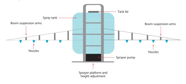
mounted tank level gauge) so that diluent level can be assessed. The lower section of the tank should have a sump to ensure that the herbicide mixture (or water with direct injection systems) is directed to the delivery system without interruption. An agitator should be used to maintain the homogeneity of the mix.
