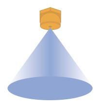
Narrow angle solid cone nozzles are better suited to applications that require spraying through deep or dense foliage than hollow cone nozzles. Wide angle solid cone nozzles may be used closer to the ground than narrow solid cone nozzles, which helps to minimise drift.
