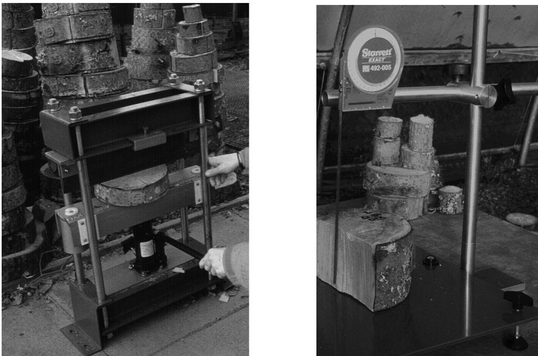
Figure 3: The first picture is an instrument which splits the logs in half and the second is a protractor, an instrument that measures spiral grain angle [2].
