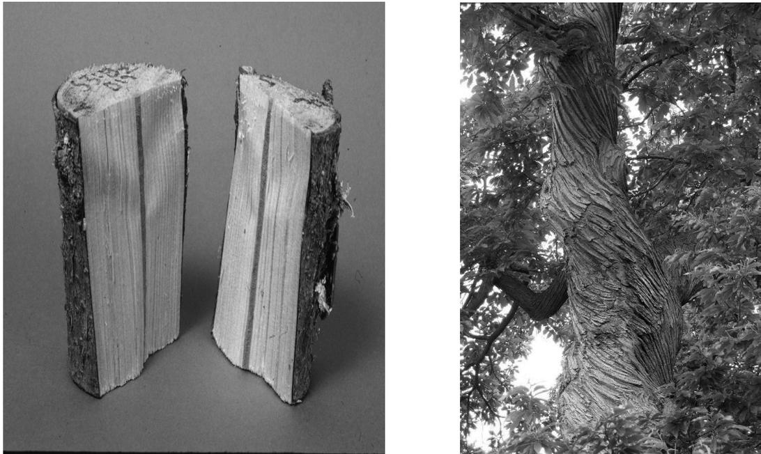
Figure 1: The picture on the left shows a split disc which uncovers the inner spirality [1], and the one on the right displays how spiral grain appears in the external part of the tree [2].
