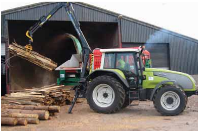
Chipper producing fuel from slab wood
