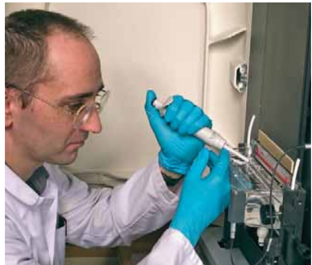
Figure 1 Loading samples of amplified DNA from black poplar on to a gel in a Licor sequencer.
