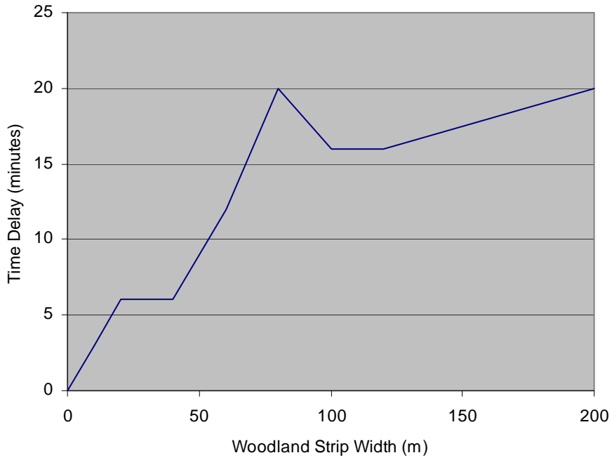
Figure 10 The effect of varying the width of woodland across the floodplain on peak flow lag time.
