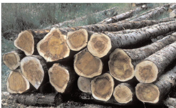
Figure 8 Discolouration and decay in logs infected with Heterobasidion annosum .
