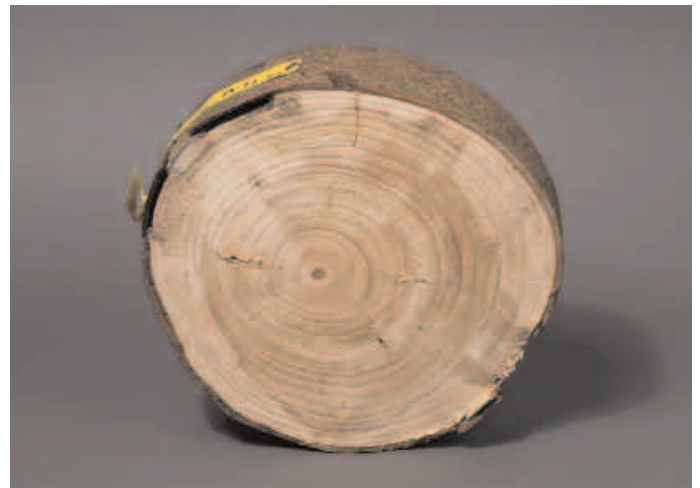
Figure 2 Internal radial cracking in the wood of Sitka spruce damaged by drought.
