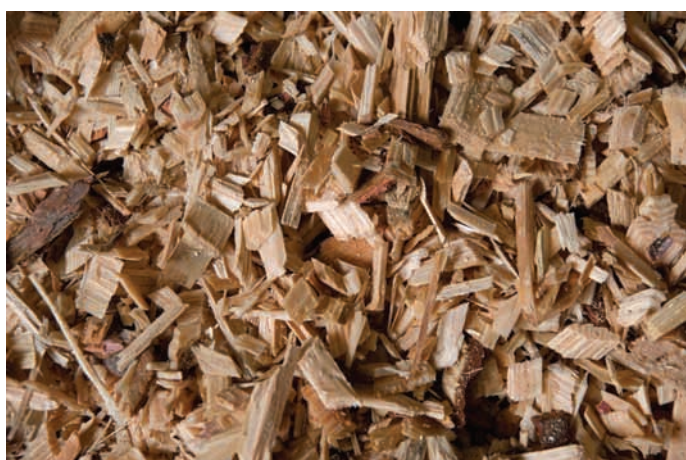
Figure 2 Woodchips are used to fuel CHP plants and biomass boilers.
