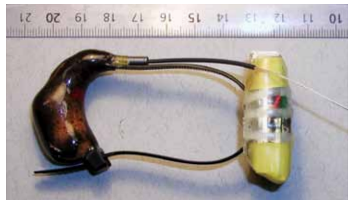
Figure 3 VHF radio and GPS collar.
