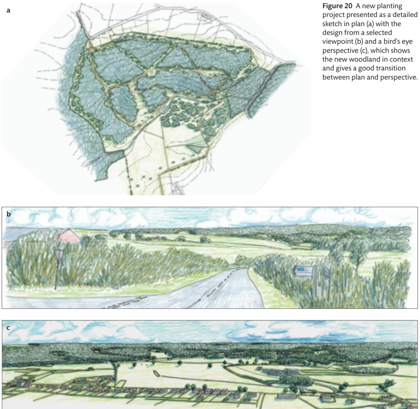
**Figure 20** A new planting project presented as a detailed sketch in plan (a) with the design from a selected viewpoint (b) and a bird's eye perspective (c), which shows the new woodland in context and gives a good transition between plan and perspective.
