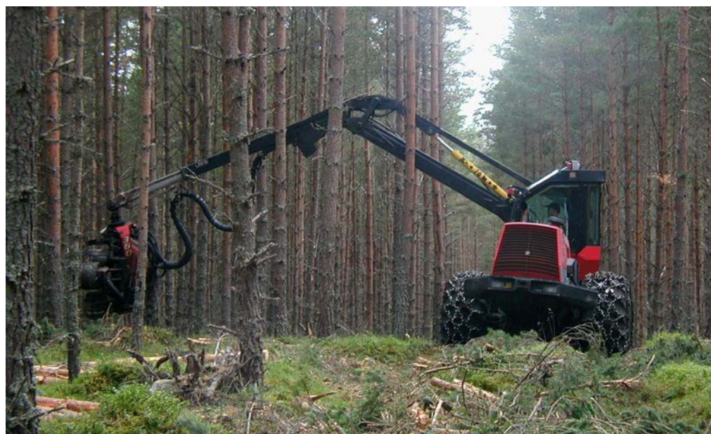
Figure 6 Crop data from harvester heads can be used to estimate the GYC of a second rotation.
