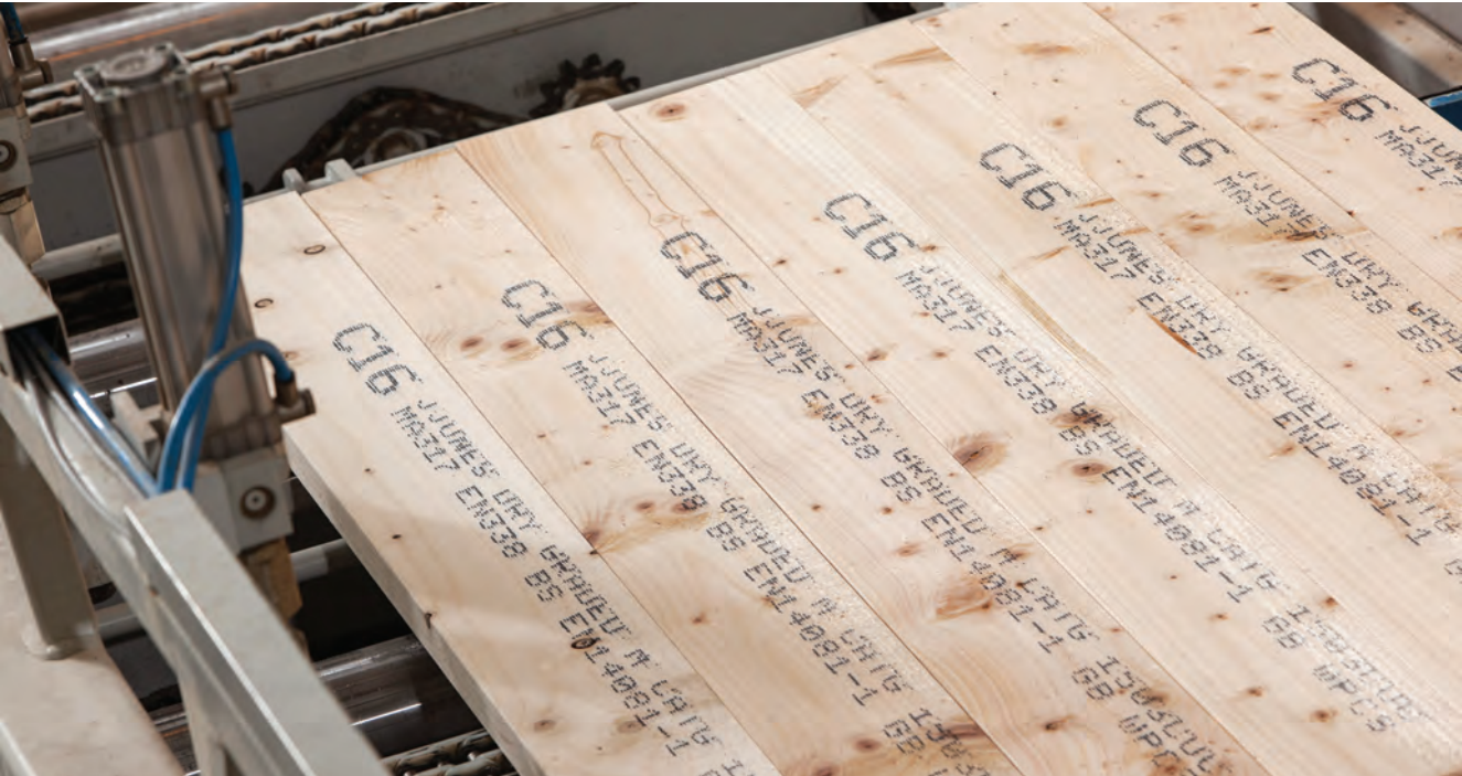
Figure 31 Machine graded spruce that has been piece marked with its strength class (C16) and other relevant information.
