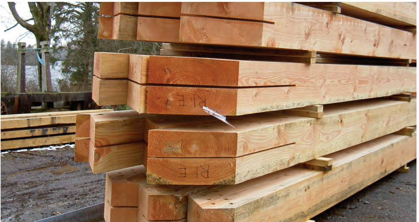
Figure 30 Visually graded Douglas fir timbers with their ends prepared for receiving metal connectors.
