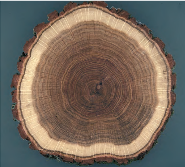
Figure 34 Cross section of an oak log with the heartwood and sapwood clearly distinguishable.
