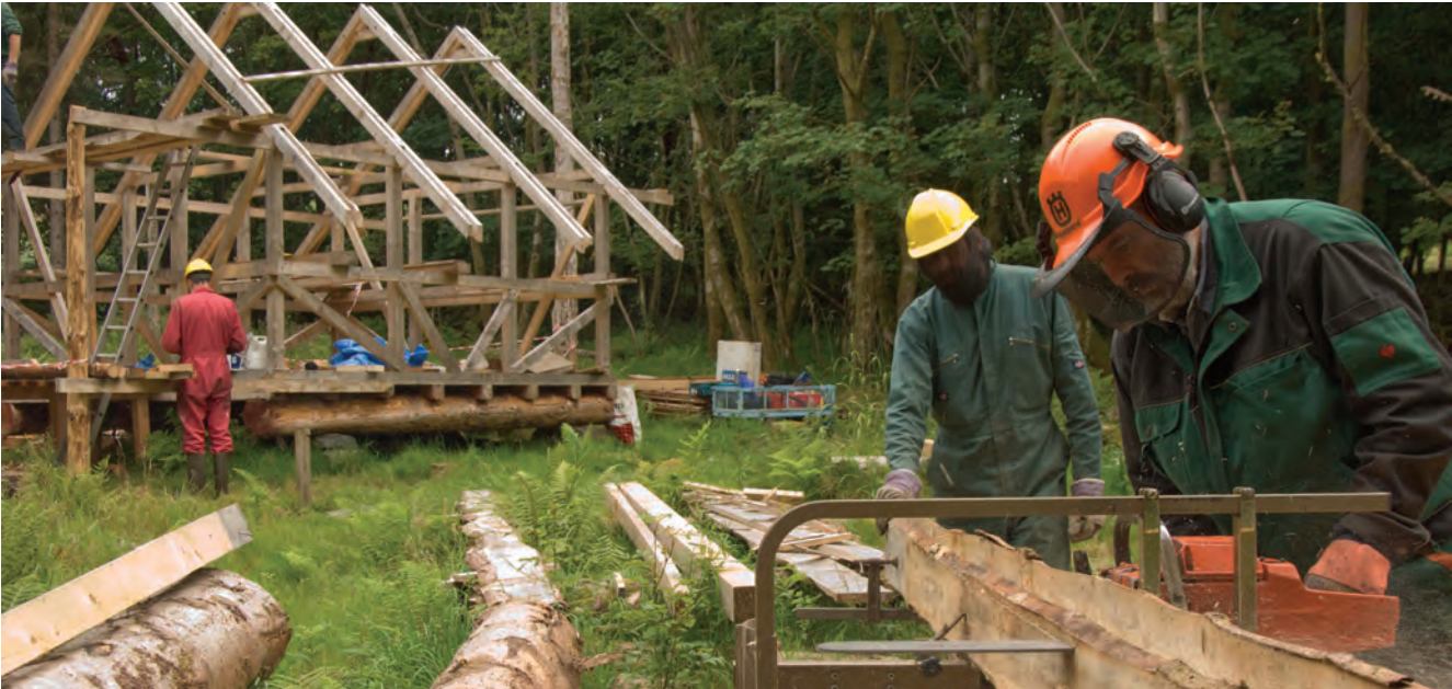
Figure 45 A chainsaw mill being used to saw timber for a small community building.
