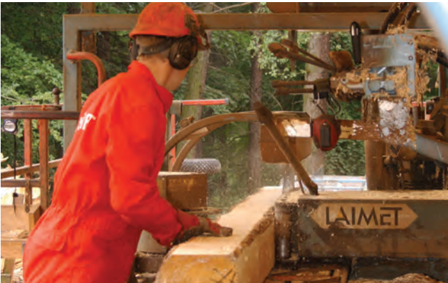
Figure 44 A mobile saw being used to process timber on-site.
