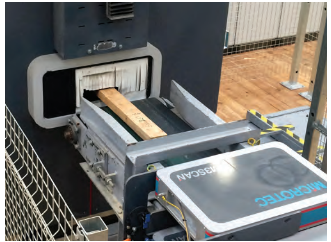
Figure 28 Timber bring machine strength graded at a sawmill.
