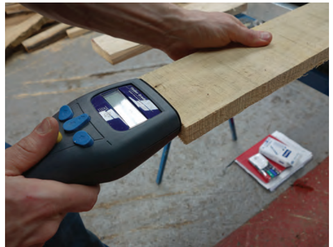
Figure 29 A hand held acoustic grader being used to measure a piece of timber.
