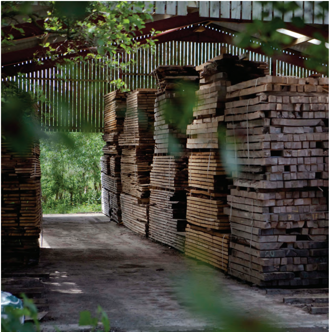
Figure 21 Air drying shed at a furniture maker in Cumbria. Air drying is mainly used to reduce the moisture content of hardwood timber prior to kiln drying.
