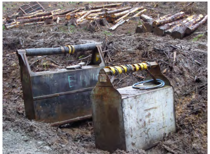
Figure 32 Containers placed on uneven ground are more liable to tip over, resulting in serious spillage.
