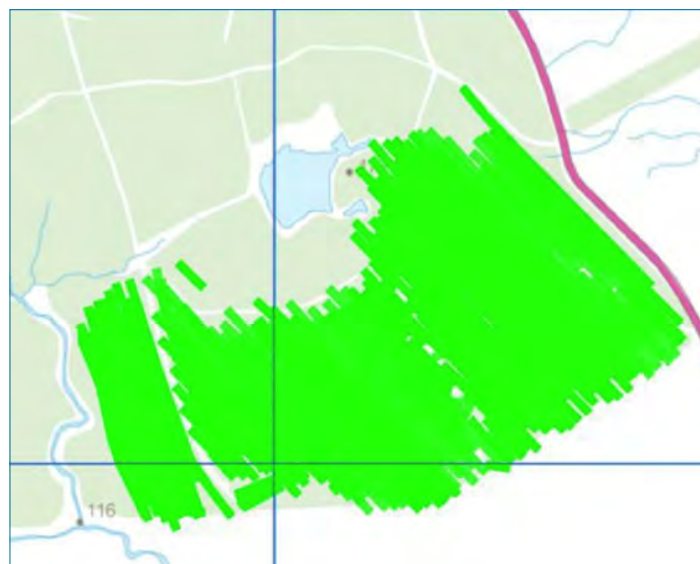
Figure 11 This spread pattern recorded by a helicopter guidance system shows that the use of map co-ordinates to guide aerial fertiliser application can reduce the risk of treating buffer areas.
