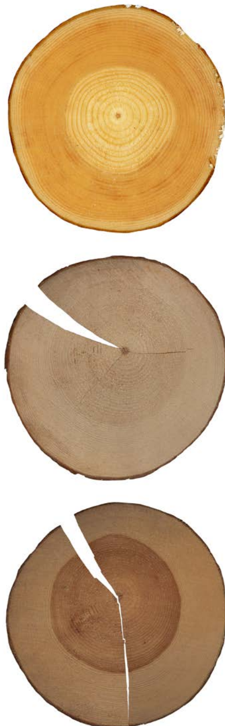
Figure 2.6 Heartwood and sapwood of freshly cut Scots pine from northern Scotland, where the heartwood is visibly drier (top); on drying this difference is visible, but less pronounced (middle); however, after continued exposure to ultraviolet light, for instance from the Sun, then heartwood will eventually become darker in colour (bottom).
