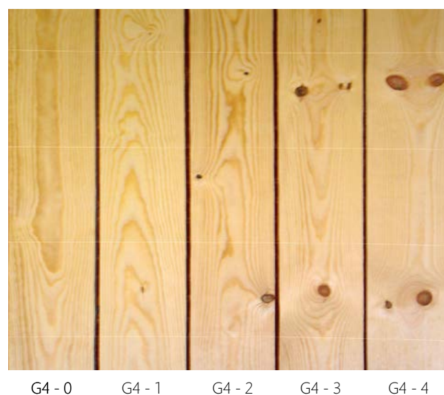
Figure 3.1 Appearance grades of softwood timber. The highest grade is shown on the left and the lowest grade on the right.
