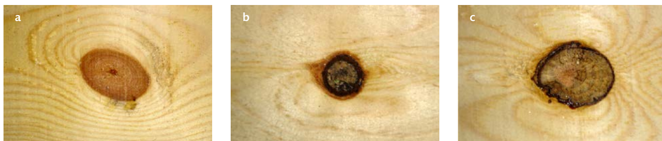
Figure 2.9 (a) sound knot; (b) dead or partially inter-grown knot; and (c) encased or bark ringed knot.
