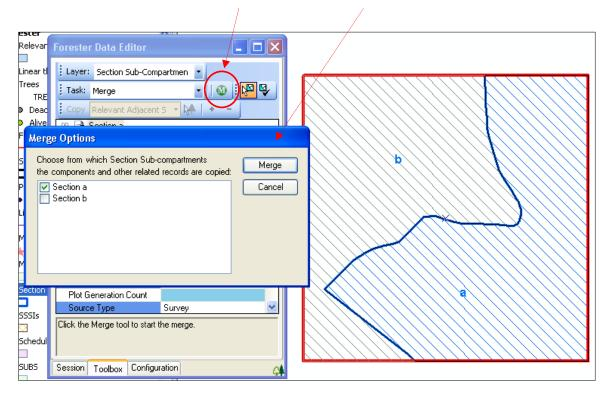
In the "Merge Options" box, place a tick against the Section(s) to copy data across from (obviously this is only relevant where the Sections already contain some Component data). Then click on the "Merge" button.
