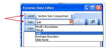
Click on the "Select Features" button to the right of the Task box, then left-click **in** the Section to be split. The chosen Section is now highlighted in blue hatching.
