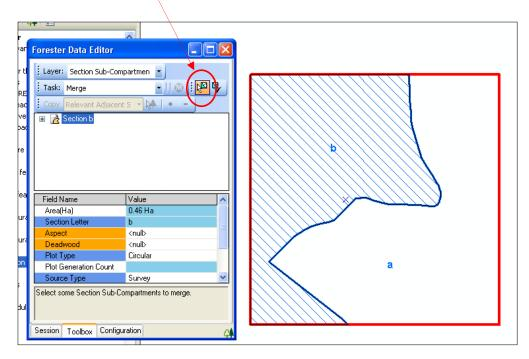
On the keyboard, hold the Shift key down and left-click in the Section that is to be merged with the first Section. Both Sections are now highlighted in blue and grey hatching, and the Section names are listed in the Forester Data Editor window.
