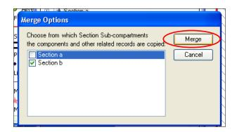
In the above example, Sections A and B will be merged into one, and the original Section B Component data will be copied across to the newly merged Section.
