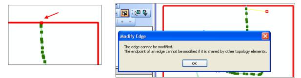
Nodes can be moved using the Slide Node Tool. See 5.5 Slide Section Boundary Nodes, for instructions on how to do this.
