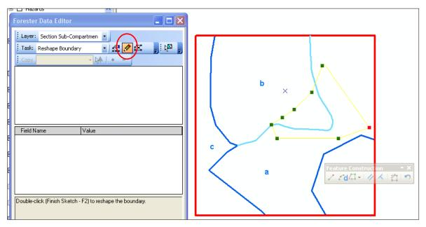
To amend the re-shape, press "Control and z" on the keyboard and this will undo the last vertex. Repeat until back at the start of the drawing.
