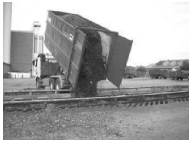
Figure 25: Off-loading system for wet wood chip at Enköping.
