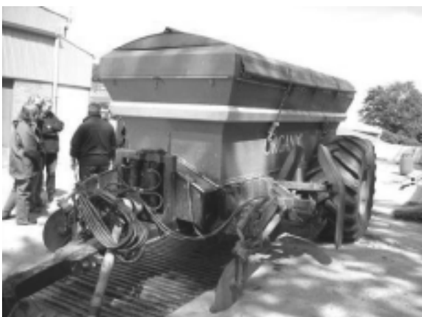
Figure 22: Organic sludge injector used at Brook Hall Estate.
