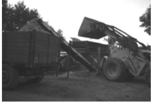
Figure 14: Screening system for willow chip.
