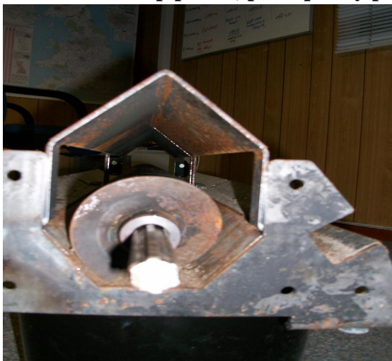
Auger too small allowing pellets to clog up inside
