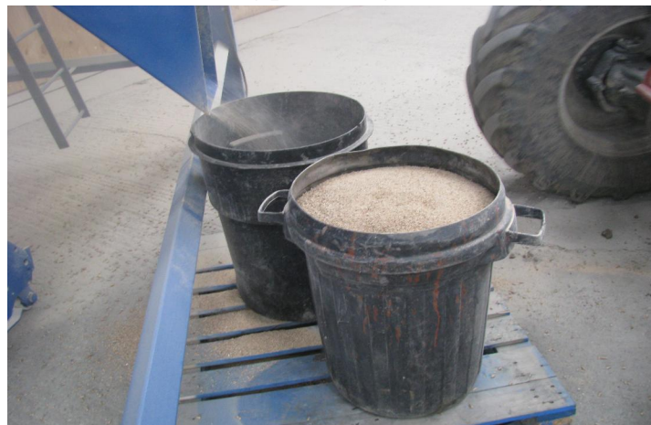
Dust and Fines Extracted at Screening Plant
