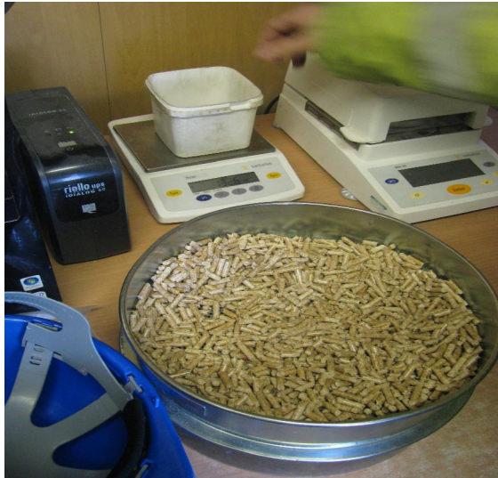
Pellets Being Tested for Durability and Fines Content
