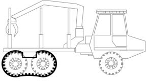
Stage 5 The track fitting tool is placed on one side of the track and a ratchet used to tighten the track, it is then connected and the 'C' staple removed. The process is repeated on the other side
