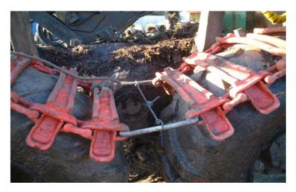
6. The forwarder operator or second person then places the track fitting tool on one side of the track (Plate 4), it is tensioned up using a ratchet socket and the C-shaped staple is removed. A long or short joining link is then inserted and the connection bolts are attached and secured. This process is repeated for the other side of the track.
