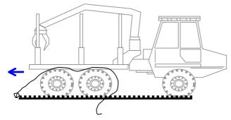
Stage 2 The operator reverses onto the track. He attaches a rope to one track end, lifts it over the machine wheels and tracks it into second wheel for traction grip
