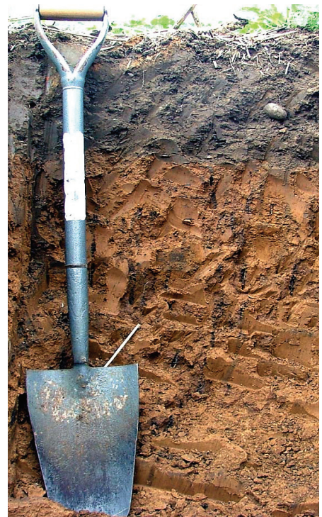
Figure 5 Soil profile pit: useful for studying soil types with depth, investigating rooting depths and sampling soils for chemical analysis.
