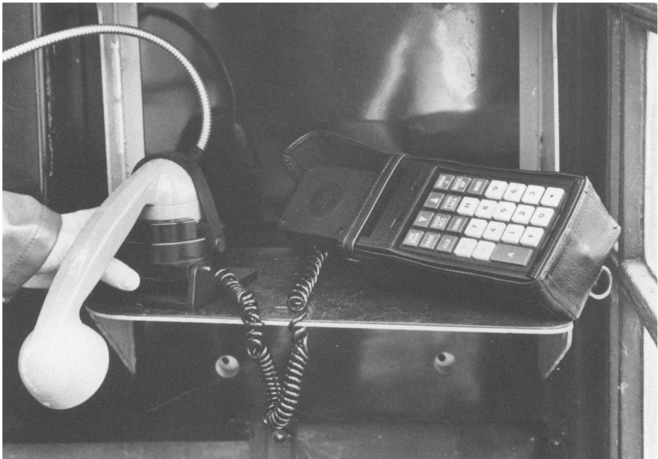
Figure 14. An MSI 88 attached to an acoustic coupler for transfer of data over a telephone line. (B9339)
