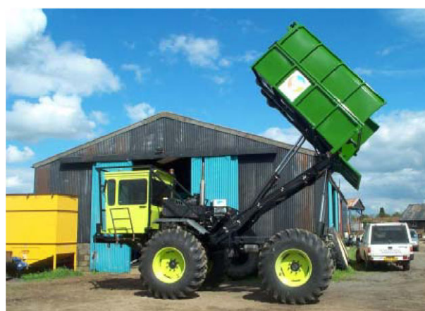
Figure 1 Completed chip shuttle, showing high tip bin mechanism in action
