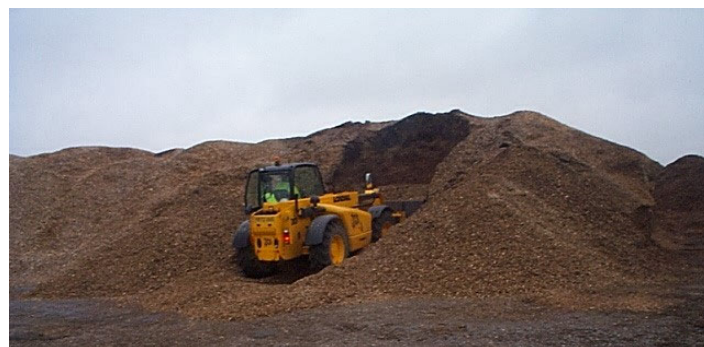
Figure 2. Interim sampling - using a teleporter to make a vertical face in the forestry residue pile
