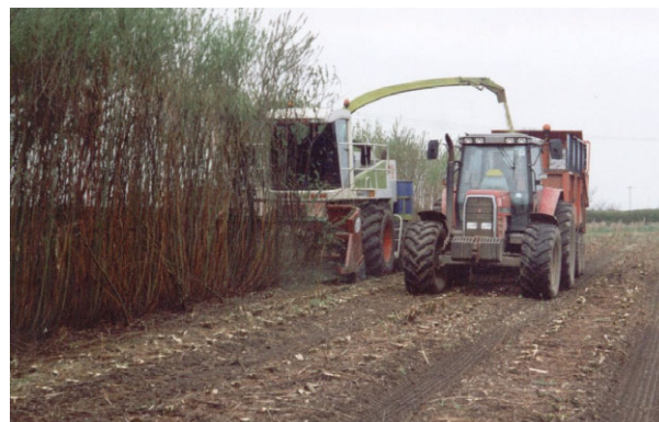
Figure 1 The cutting head mounted on a Claas forage harvester
