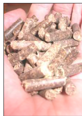
Highly compressed heather pellets, 2010
