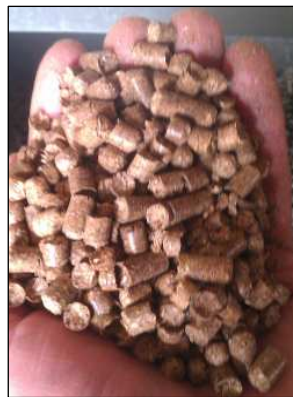
Low durability heather pellets
