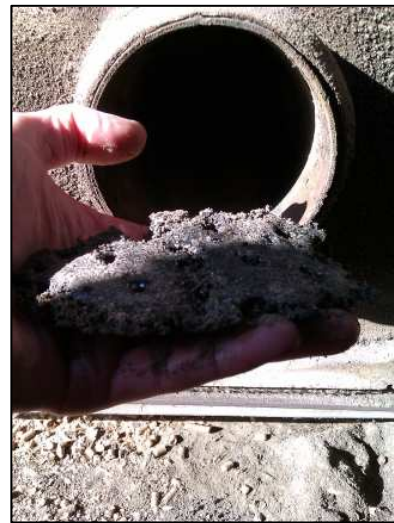
One week's Clinker from heather pellets
