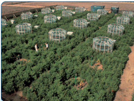
Open-top chambers used to investigate the effects of ambient air pollution on tree growth.
