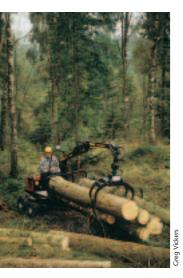
Extraction equipment, such as this Alstor mini-forwarder, may be useful where there are sensitive ground conditions or narrow trackways.
