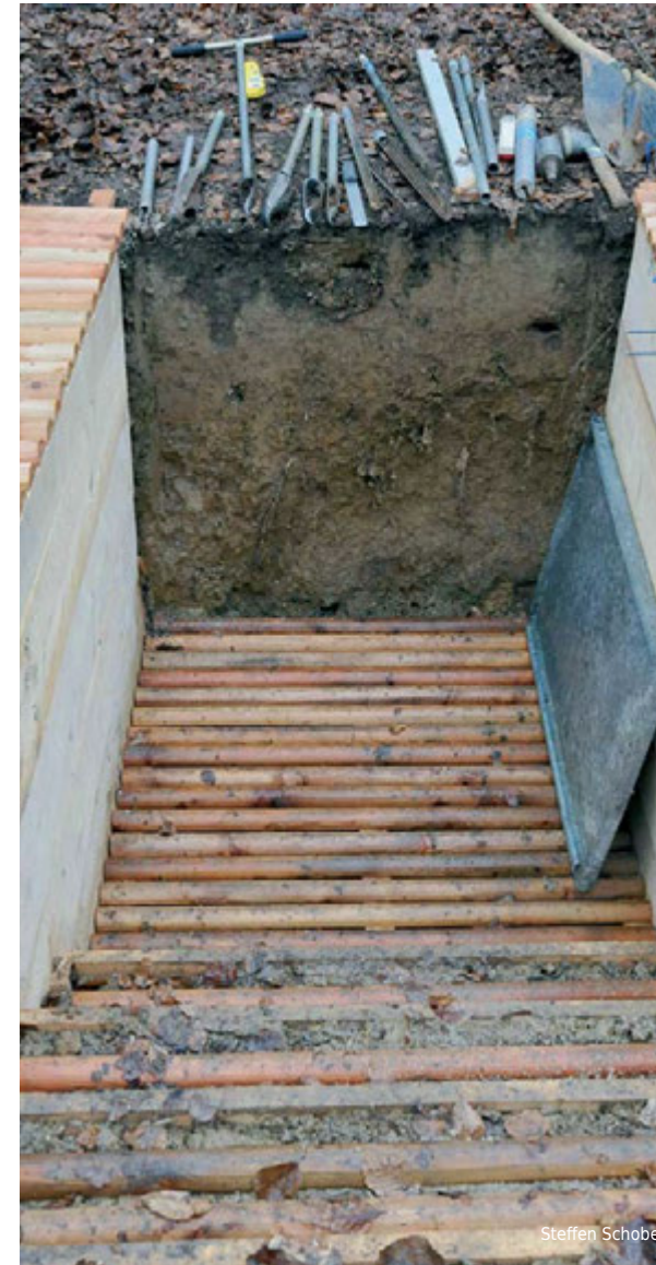
Permanent soil sampling plot and installation of a soil moisture sensor (tensiometer) in Freising, Germany.
