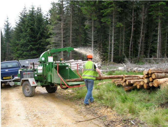
Figure 3 Manually loading the Bandit 90W chipper with the shorter lengths of Sitka spruce
