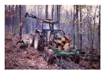
crops Although work outputs for agricultural tractor forwarders<sup>1</sup> are generally much lower than for purpose built forwarders, their low capital costs make final extraction costs competitive with large scale equipment.
