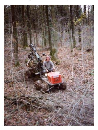
Terrain factors prevented the wire loader from getting timber to the official stacking area and it was unloaded in the wood. The other 3 forwarders managed to extract to the stacking area.
