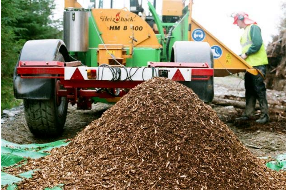
Plate 2 Material produced when chipping 100% brash
