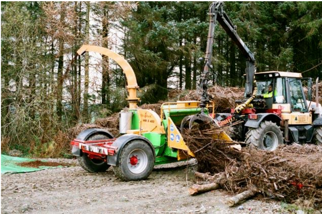
Plate 1 Chipper and loader
