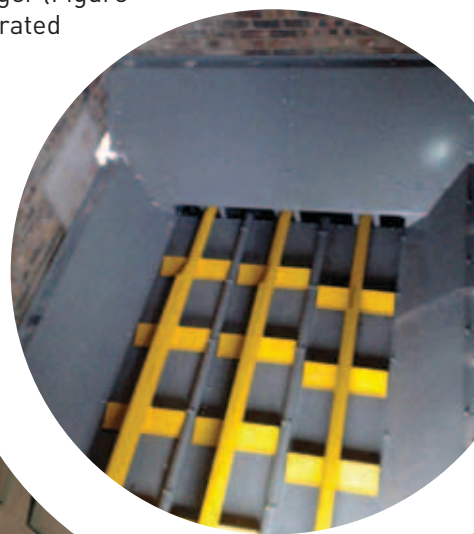
Figure 9 Chip store using a walking floor (Ashwell Engineering Ltd).
